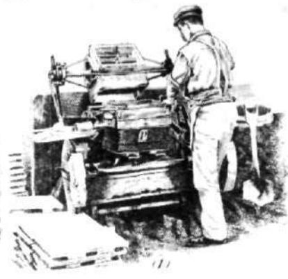
Operating a moulding machine, c. 1900. International Correspondence School. Machine Molding . . . Metropolitan Toronto Library Board.
